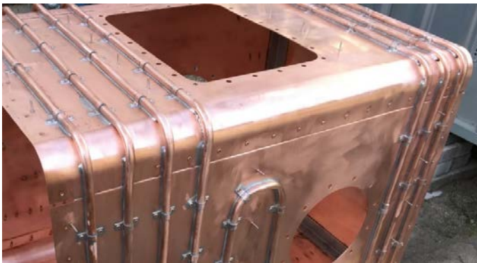
Figure 4a: Thermal shield of the CCC cryostat. During the assembly, two copper tubes surrounding the room-temperature UHV-beamline are inserted in the holes (bottom right) on either side of the shield.
