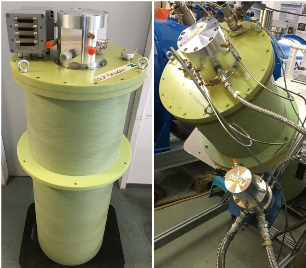
Figure 5: (Left) Side view of the LHe cryostat for magnetocardiography with the cold head mounted in the centre of the lid and the SQUID sensor connection boxes on the left side of the lid. (Right) Cryostat tilted at 45 degrees in cold condition (without SQUID's).
