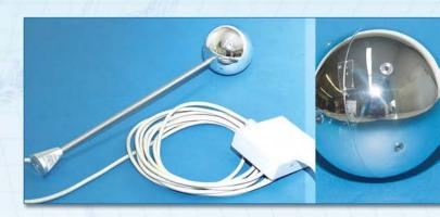
Measuring System for Determination of Three-Dimensional Air Flow Conditions
