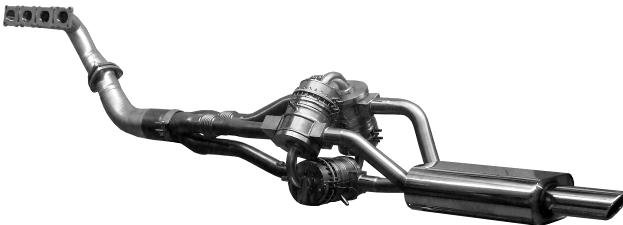
Figure 3: Integration of the thermal engine in the exhaust gas system
