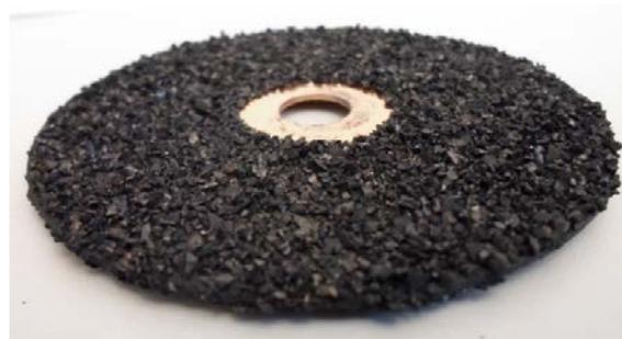
**Figure 1:** Prepared cryopanel coated with activated charcoal (carbon elements)
