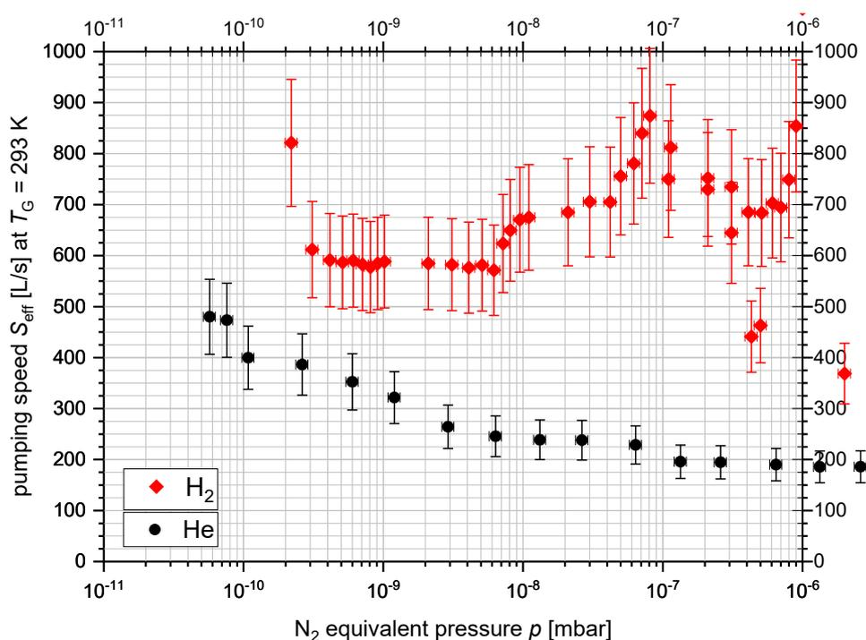
**Figure 8: Pumping speed measurements of the cryosorption pump (GSI)**
