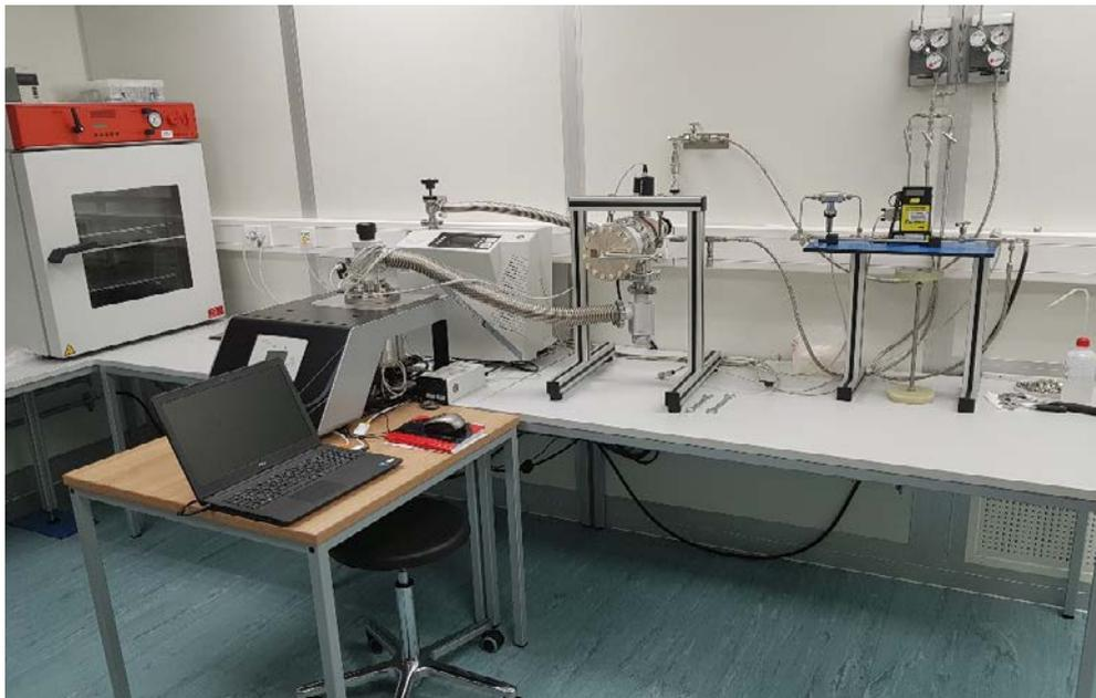
**Figure 4: Test rig for mass flow and pressure loss measurements**
