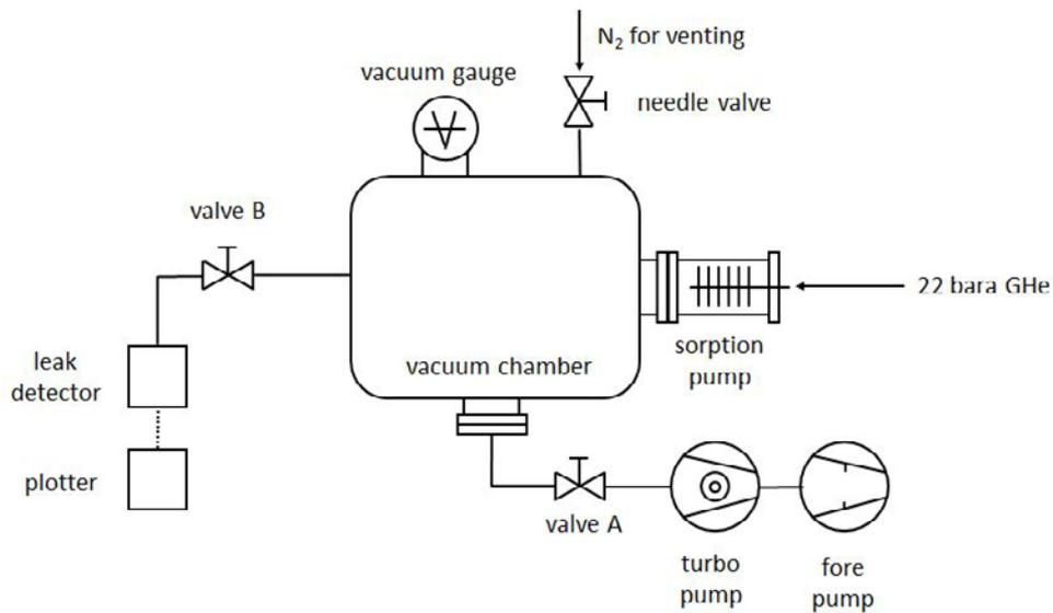
**Figure 3: Schematic drawing of the test rig for mass flow and pressure loss measurements**
