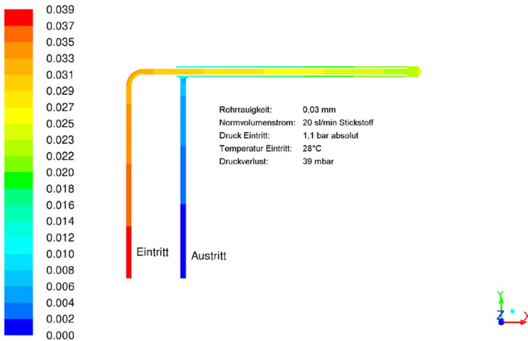
**Figure 5: CFD simulation of pressure loss inside the cooling tube**
