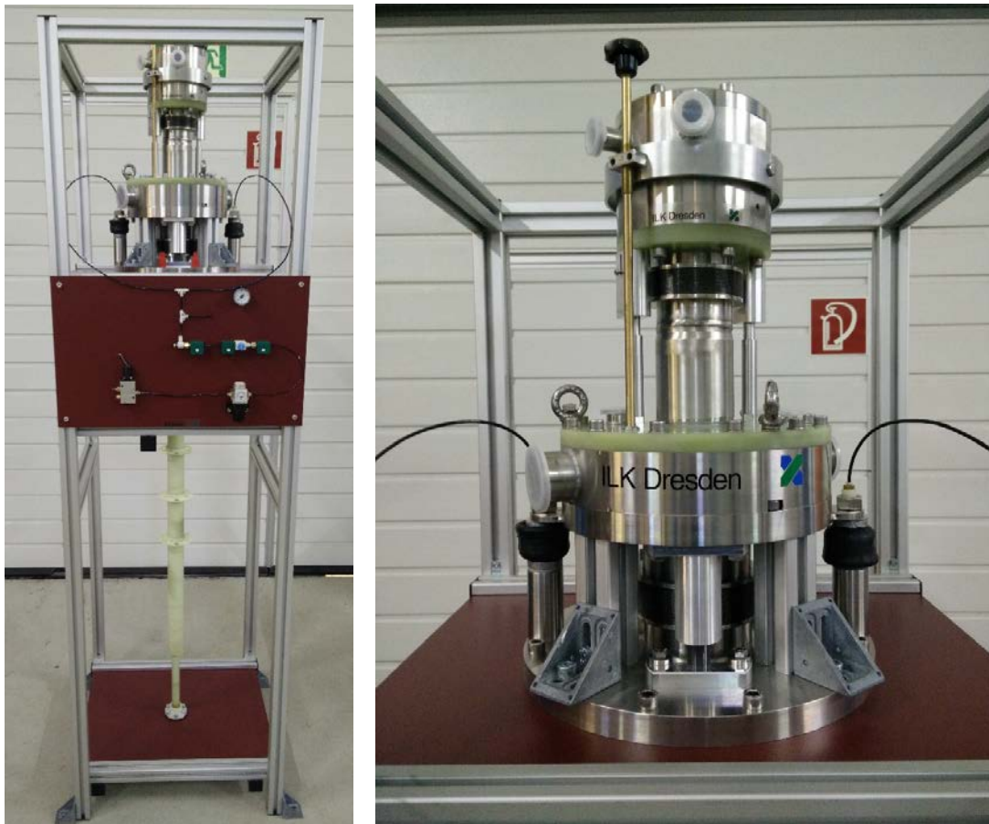
Figure 4: Non-metallic variable temperature insert (VTI) for a helium cryostat
