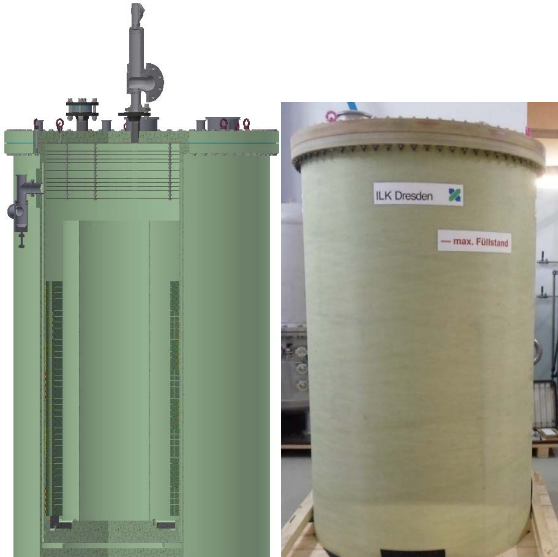
Figure 1: Cryostat for HTS cooling (left: schema including mounted safety valve, right: finished cryostat)
