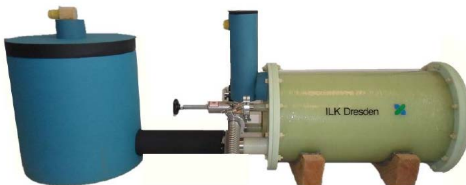
Figure 3: Non-metallic cryostat for small-animal MRI
