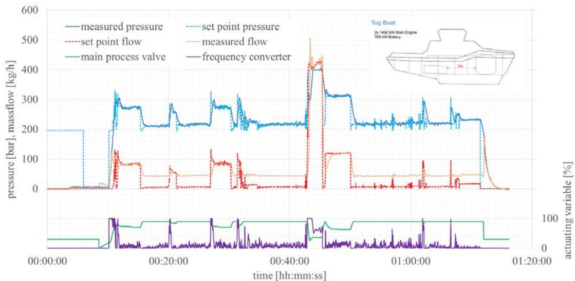
**Figure 3: test results of simulated tugboat operation**
