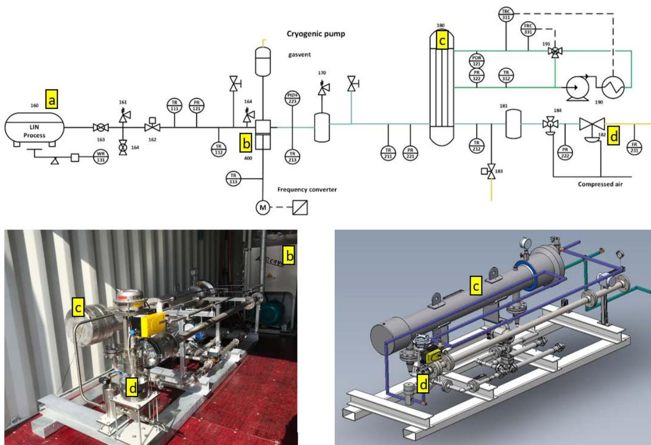
Figure 1: PID, 3D model and built system with the main components: a – LIN Tank, b – cryogenic high pressure pump, c – double tube safety heat exchanger, d – main process valve
