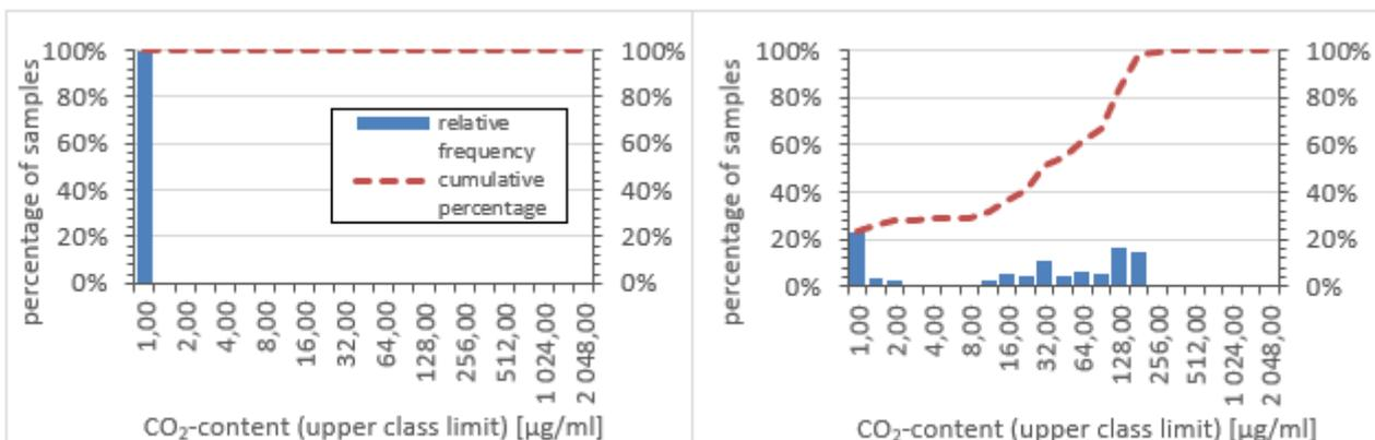
**Figure 2: Comparison of the CO<sub>2</sub> content for 96 vials each from two different manufacturers.**
