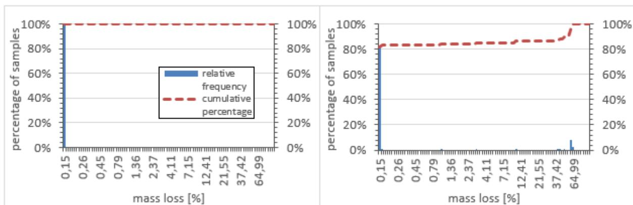
**Figure 4: Comparison of the mass loss after gravimetric leak test for 96 vials each from fresh and thermally stressed tubes**
