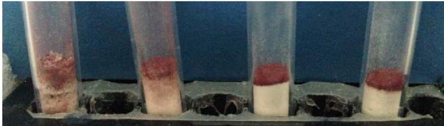
**Figure 3: Result of the LN<sub>2</sub> leak test. From left to right: residual pressure and mixing effect positive, mixing effect positive and residual pressure negative, mixing effect and residual pressure negative (tight vial), mixing effect negative and residual pressure positive.**
