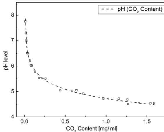
**Figure 1: Fitted correlation between measured pH value of the sample and CO<sub>2</sub> content of the absorption buffer**
