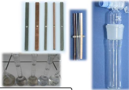
► ILK tested at 250 °C NH3/Water in high-pressure autoclaves last year
